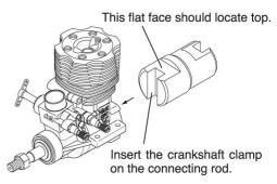
72530510 (exclusively for 91) and 71530520 (exclusively for 91/105) cannot be used with the GT15HZ. If they are used with the GT15HZ, piston skirt will be broken or damaged.
